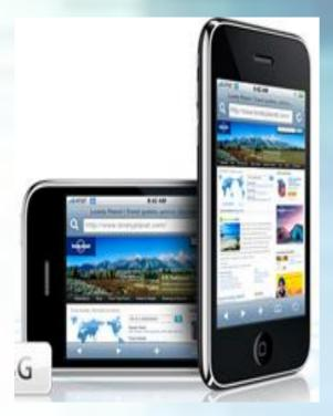
The appearance of the second generation, iPhone 3G has no big difference with the previous one. The new functions added in are the GPS, which allow users to use Geo-tagging to record the information. Also, the memory size has increased from maximum 8GB to 16GB.
